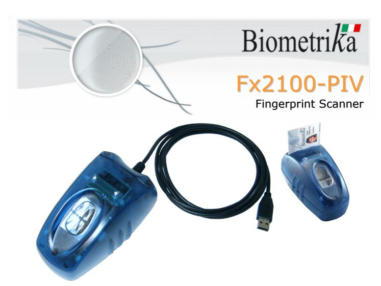
Fx2100 is a FTIR optical fingerprint scanner, which, thanks to its powerful CPU is capable of performing in hardware several useful tasks, thus improving security, efficiency and usability. The accurate optical design allows high quality images to be captured and a large finger area to be sensed.
